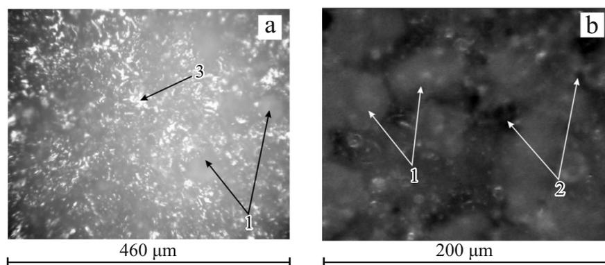
Fig. 2. Morphology of the Cu-HA coating: 1 — particles of sprayed powder, 2 — open pores, and 3 — titanium base.
