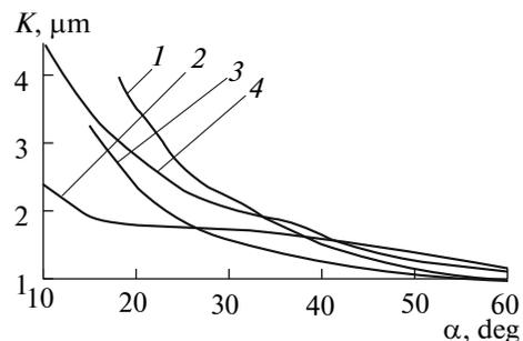
**Fig. 3.** Dependence of  $K$  on the setup angle  $\alpha$  when  $n = 2$  (1), 3 (2), 4 (3), and 5 (4);  $n$  is the number of the harmonic.
