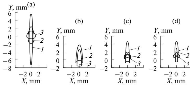
**Fig. 2.** Trajectories of the blank’s center: (a) second harmonic; (b) third harmonic; (c) fourth harmonic; (d) fifth harmonic; (1)  $\alpha = 20^\circ$ ; (2)  $\alpha = 40^\circ$ ; (3)  $\alpha = 60^\circ$ .
