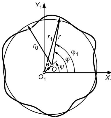
Fig. 1. Measurement scheme in a roundness gauge.
