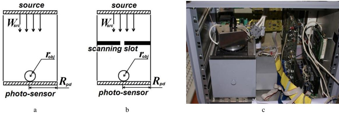
**Figure 1.** Scheme of edge scanning optical microscope (a,b) and measuring part of experimental setup (c)
