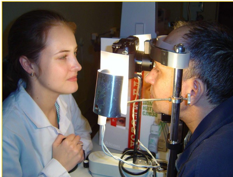
Figure 7: Experimental setup for in vivo registration of digital images of human irises
